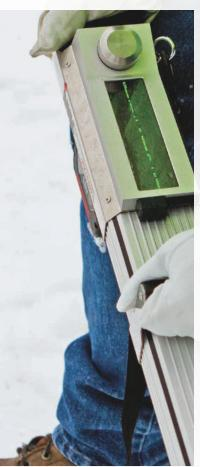
The **PD500 Resistograph** allows the user to identify soft spots and voids inside the wood to determine a utility pole's strength.
